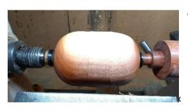
OK, box mounted, now turn the outside and sand to match the ends
