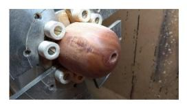
At this stage, fine turn the ends of both pieces and sand up to  $600\,$  minimum.
