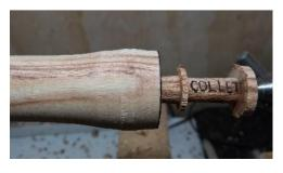
You can see the collar that stops the timber going too far into the collet. I also leave the end where the live centre touches larger than 3/8in. This stops the live centre splitting the 3/8in spigot. I cut this off before insertion into the collet chuck.
