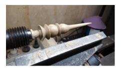
Sanded and 1 coat of Spraylac. Note undercut of pedestal. This is done to match the curvature of the lid of the box. Stem is sized to 3/8in and cut off to fit
