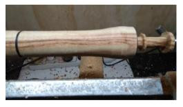
Next, at the live centre end turn down to 3/8 in for collet chuck. Note, if you don't have a drawbar collet chuck, and you are using pin jaws or long nose jaws, then you only need the size for your own jaws.
