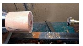
I have parted the cylinder, and chucked the lid piece ready to be drilled out to the required depth with a forstner bit.
