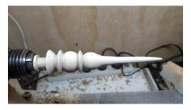
Nearly finished, just a little bit more off towards the tip, and the pedestal underside to be cut
