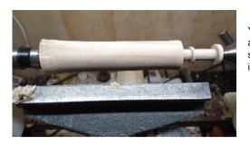
You can see the collar that stops the timber going too far into the collet. I also leave the end where the live centre touches larger than 3/8in. This stops the live centre splitting the 3/8in spigot. I cut this off before insertion into the collet chuck.
