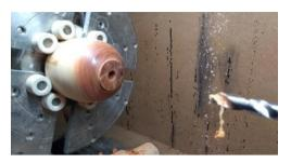
Hole drilled, depth approx. 5mm, depends on how close you have turned to the bottom of your pieces.
