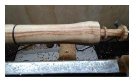
Next, at the live centre end turn down to 3/8 in for collet chuck. Note, if you don't have a drawbar collet chuck, and you are using pin jaws or long nose jaws, then you only need the size for your own jaws.
