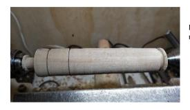
Now mounted in collet chuck, and live centre brought up. Markings made for flanges
