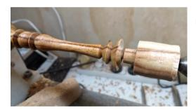
Sanded to 240 just for this demo, Spraylac. Cut off marked to go into base of box.
