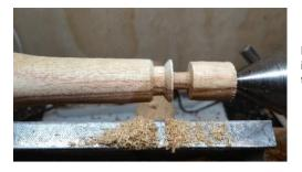
Now mounted in collet chuck, and live centre brought up. A 3/8in spigot is now recessed into the cup where the stand will go into the bottom of the box. This will be trimmed to fit later.
