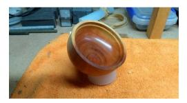
Drilled out, flange made, polished, the outside roughly turned, and parted off. The reason for only roughly turning the outside will be explained later.
