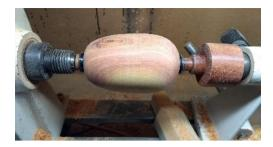
Shape finished, joint and body all sanded to 600 to match the ends that were previously done.
