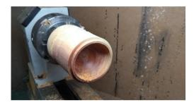
Base mounted, drilled out, flange matched, and ready to polish inside
