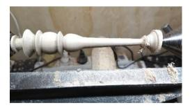
Shape nearly completed, tip to be thinned down, and ball and flanges made crisper with 1/4in skewchigouge
