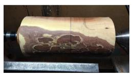
Select your timber, rough down to a cylinder, and cut spigots on each end for a normal 100mm chuck. Depending on your design, mark where you will part, some boxes will have different sized lids.
